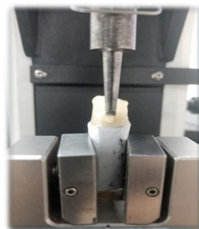
Figure 4: Measuring shear bond strength in UTM machine
