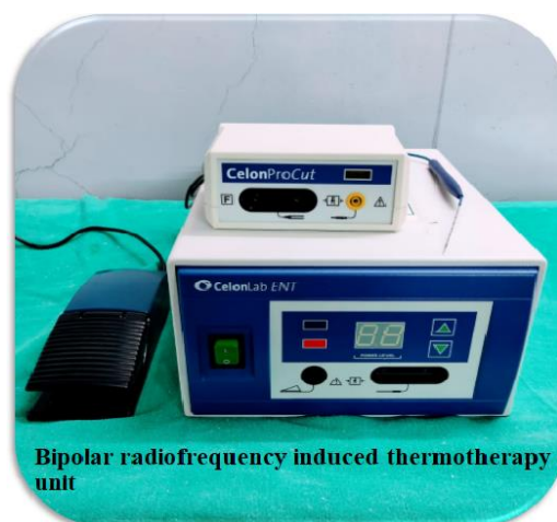
Figure 1: Bipolar radiofrequency induced thermotherapy (RFITT) unit and needle electrode
