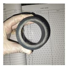
Fig.2- PVC stopper with circular opening
