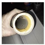
Fig. 5 PVC pipe with 2 layers of double-sided tape
