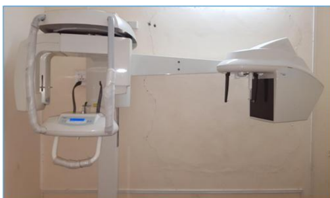
Fig. 1 Digital Cephalostat machine Carestream CS 8000c
