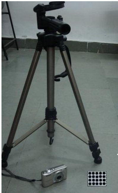
Illustration 3.1: Shows instruments (tripod stand, camera, markers) for measuring the cranio-vertebral angle
