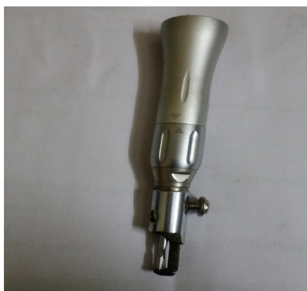
Figure 5 Coustom made dental hand piece with dura guard and burr-side view
