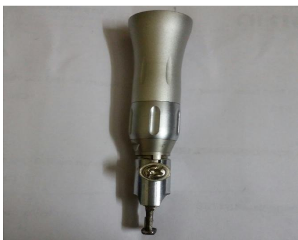
Figure 4 Dental hand piece with custom made dura guard - front view
