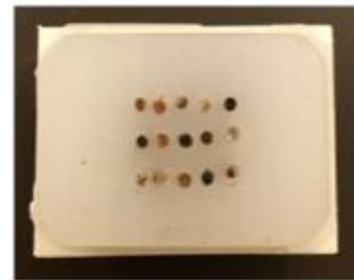
Figure E: Finished TMA using Prefabricated recipient block technique (Kononen et al)
