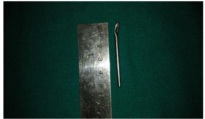
Fig 5 Retrieved broken part of needle
